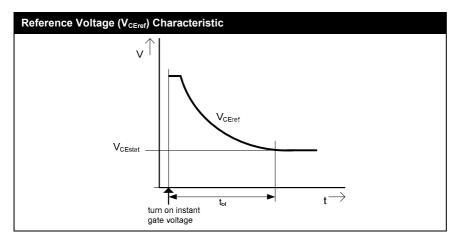
After  $t_{bl}$  has passed, the V<sub>CE</sub> monitoring will be triggered as soon as V<sub>CEsat</sub> > V<sub>CEref</sub> and will turn off the IGBT. The error memory will be set, and the output PRIM\_HOLD\_OUT changes to the HIGH state. Possible failure modes are shows in the following pictures.
