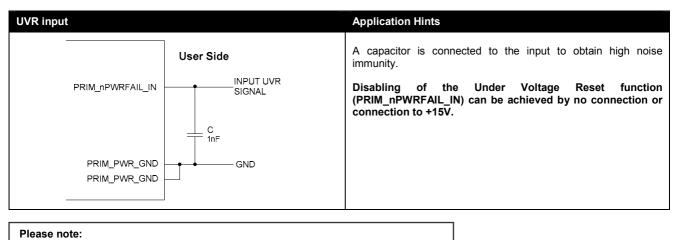
Do not use PRIM\_nPWRFAIL\_IN to place the driver core into halt mode during operation.
